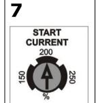
The **Start Current [150-250%]** select the initial current starting in % of Full Load Current.
