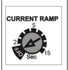
The **Current Ramp [off-15sec]** select the ramp time in secconds. The starting current ramp extends the time necessary to the soft starter to reach the current limit.
