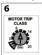
The **Motor Trip Class [0-20sec]**Select the class of alarm for the protection from motor overload. This trip class represents the time in seconds for which the motor can work with current conditions of the rotor blocked. The setting of the class of intervention engine assumes a current in conditions of locked rotor equal to 600%(6x) of Full Load Current.
