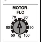
The **Motor Full Load Current [50-100%]** configures the soft starter to the related full-load current (FLC) of the motor in %.
