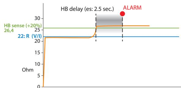
Sensitivity (HB sense) and delay (HB delay) can be varied according to the application (see parameters on pages 43-44).
