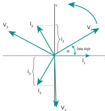
Without delay at zero crossing when  $V_1$  is to zero (projected on the X axis) the unit switch On.
