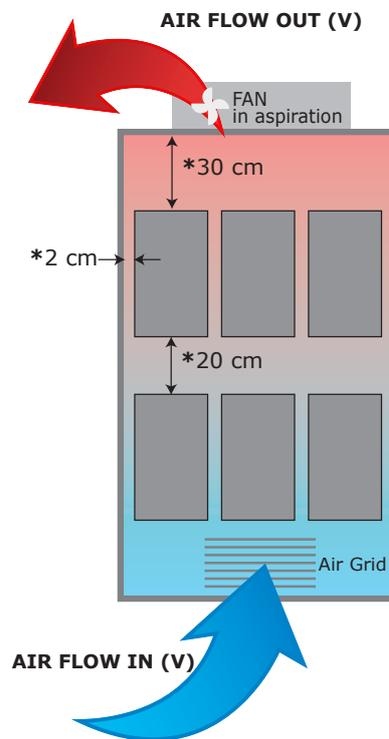
The V Air flow must be equal or more than the value calculated.
