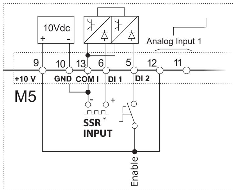
\* **SSR Input:** 4÷30Vdc 5mA Max (ON ≥4Vdc / OFF <1Vdc)
