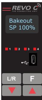
While performing the heater bakeout function, the power controller displays a message
