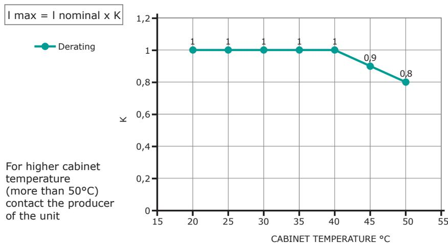
Operation at ambient operating temperature above 40°C not covered by UL®
