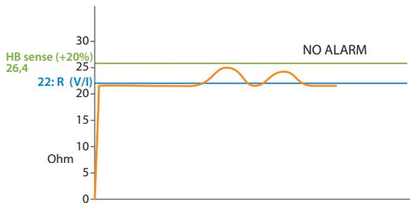
The alarm activates when the detected Runtime resistance exceeds the value of 26.4 Ohm.
