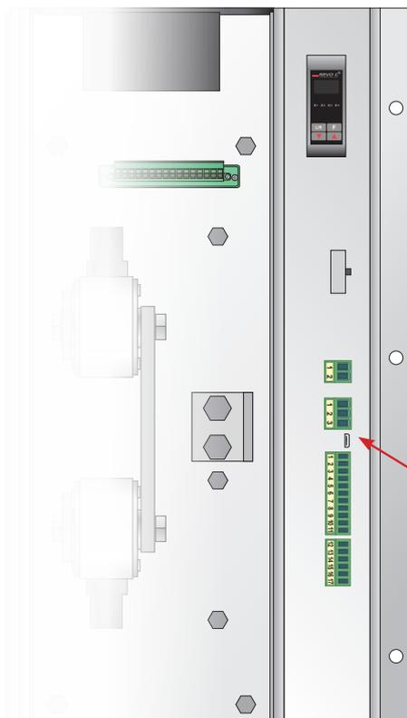
To connect the unit at the PC, it's necessary to use the micro USB 2.0 Modbus RTU cable. USB connection need a driver to work properly, you can find it from our site. However the configuration software installer will install as default the correct driver.
