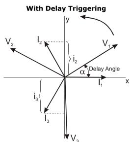
Without delay at zero crossing when V1 is to zero (projected on the X axis) the unit switch On. In this case the instantaneous value of the currents are i1, i2 and i3 and this condition, for the curve of magnetization, could generate transient over currents that can blow the fuses. With Delay Triggering the firing of the thyristor are triggered with a delay until the instantaneous value
