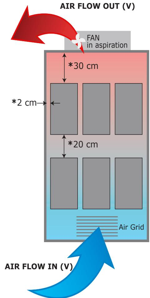
The V Air flow must be equal or more than the value calculated.
