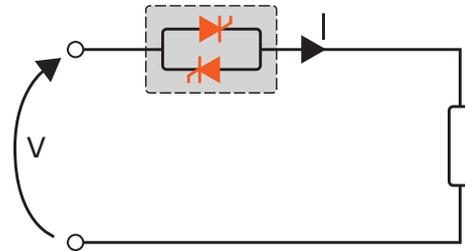
Single phase wiring with inductive load (with REVO S-1PH)
